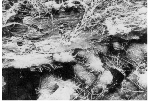
Fig. 16. Scanning electron micrograph of the anodic oxidation-hydrothermal treated hydroxyapatite coating titanium surface after 14 -days-culture ( \times 15000 ). The calified-like microspheres and network of collagen-like fibers at the surface of anodic oxidation-hydrothermal treated hydroxyapatite coating titanium (from reference 17)
