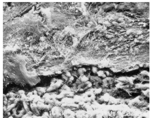
Fig. 13. Scanning electron micrograph of the anodic oxidation-hydrothermal treated hydroxyapatite coating titanium surface after 7-days-culture ( \times 5000 ) Upper area : culture cells layer and collagen-like fibers, under area the surface of anodic oxidation-hydrothermal treated hydroxyapatite coating titanium (from reference 17)
