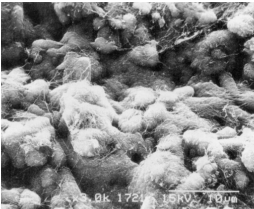
Fig. 15. Scanning electron micrograph of the anodic oxidation-hydrothermal treated hydroxyapatite coating titanium surface after 14 -days-culture ( \times 15000 ). The calified-like microspheres at the surface of anodic oxidation-hydrothermal treated hydroxyapatite coating titanium (from reference 17)
