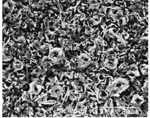
Fig. 9. Hydroxyapatite crystals precipitated \text{TiO}_2 layer
