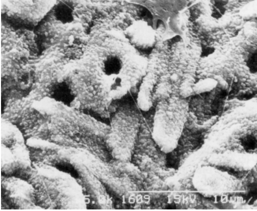
Fig. 14. Scanning electron micrograph of the anodic oxidation-hydrothermal treated hydroxyapatite coating titanium surface after 7 -days-culture ( \times 15000 ). Under area of the Fig.13, calified layer at the surface of anodic oxidation-hydrothermal treated hydroxyapatite coating titanium (from reference 17)
