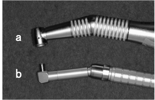
Fig. 3 Comparison of handpieces a : Micro-motor b : CO 2 laser
